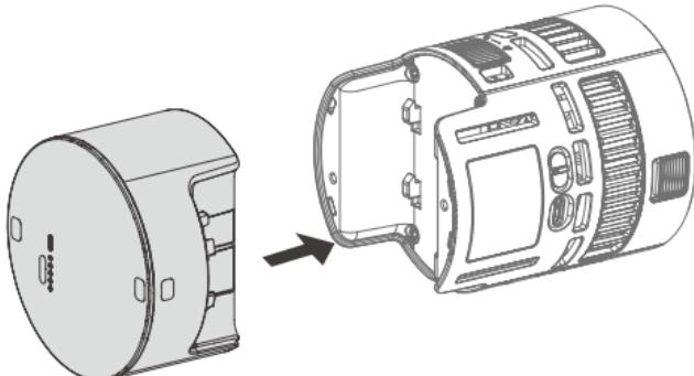
**Disassembly:** Press and hold the battery disassemble pusher, then pull the battery out to disassemble it.
