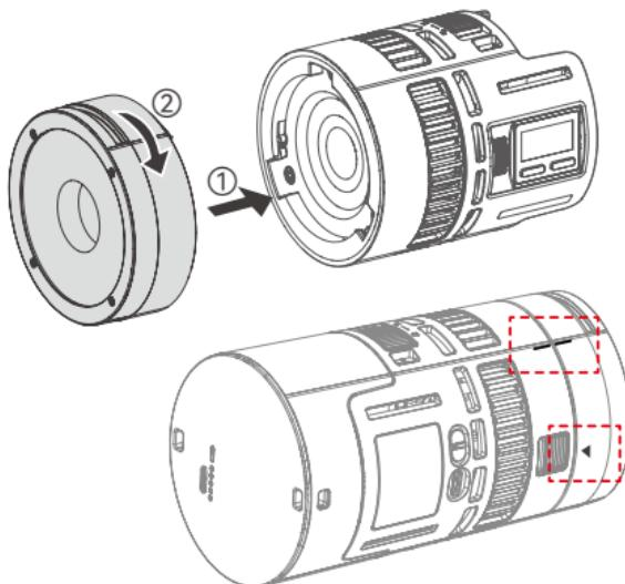
Press and hold the mount locking pusher, rotate the lens reflector anticlockwise to disassemble it.
