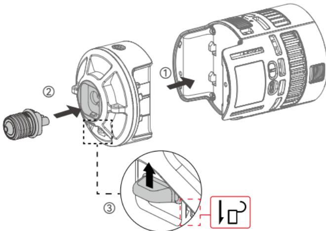
2. To disassemble, toggle the pusher until a "click" is heard to unlock and then pull out E27.
